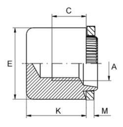
Female thread A = M12Height K = 19.0Min thread length C = 7.0Outer diameter E = 25.0Plate thickness = 2.9 to 3.1
